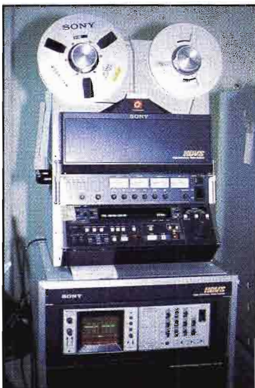
A typical HDTV production VTR appears similar to a typical 1-inch machine. The similarity is only cosmetic.
