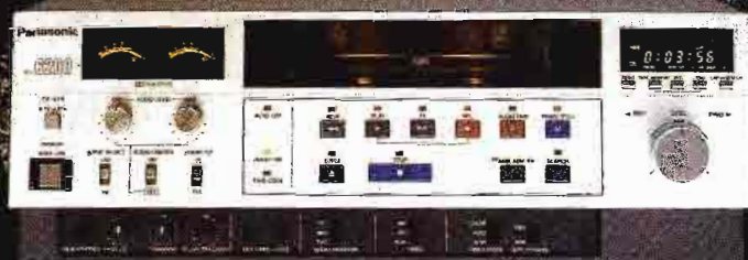
AG-6200 High performance, general purpose VHS recorder. 34-pin parallel remote interface.
